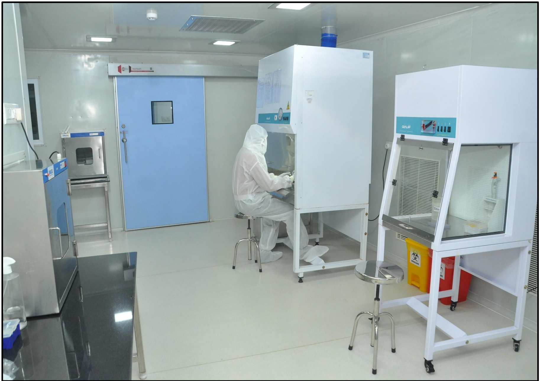
Processing of samples in negative pressure rooms to avoid contamination
